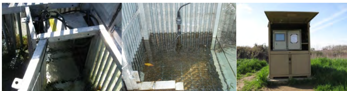
Figure 3. Left: Photograph of the Vaki Riverwatcher infrared scanner looking from upstream to downstream at the upstream side of the scanner plates. Center: Example of the riverwatcher camera and lights. Right: Tuolumne Weir Vaki Riverwatcher computer system and job box.
