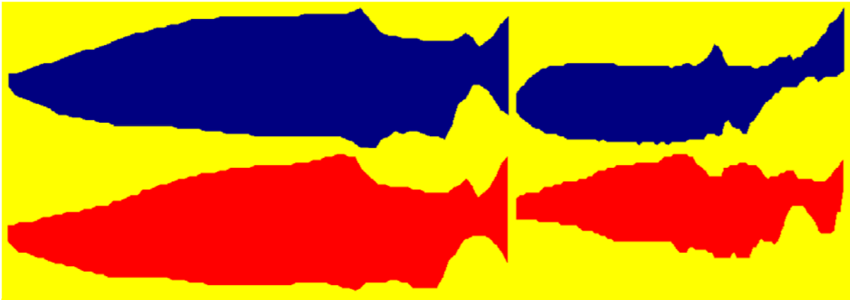
Figure 4. Example of silhouette images produced from both sets of scanner diodes (one image from one set of diodes is displayed in blue and the other is displayed in red). The left set of images is an example of a typical salmonid silhouette and the right set of images is an example of a poor salmonid silhouette.
