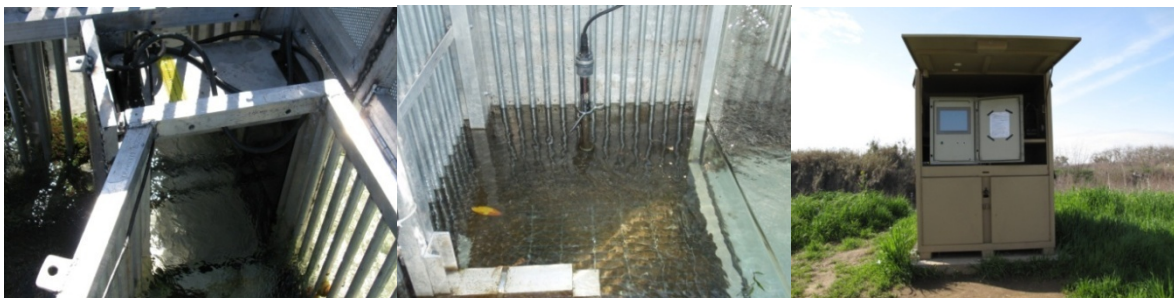
Figure 2. Left: Photograph of the Vaki Riverwatcher infrared scanner looking from upstream to downstream at the upstream side of the scanner plates. Center: Example of the RiverWatcher camera and lights. Right: Tuolumne Weir Vaki Riverwatcher computer system and job box.
