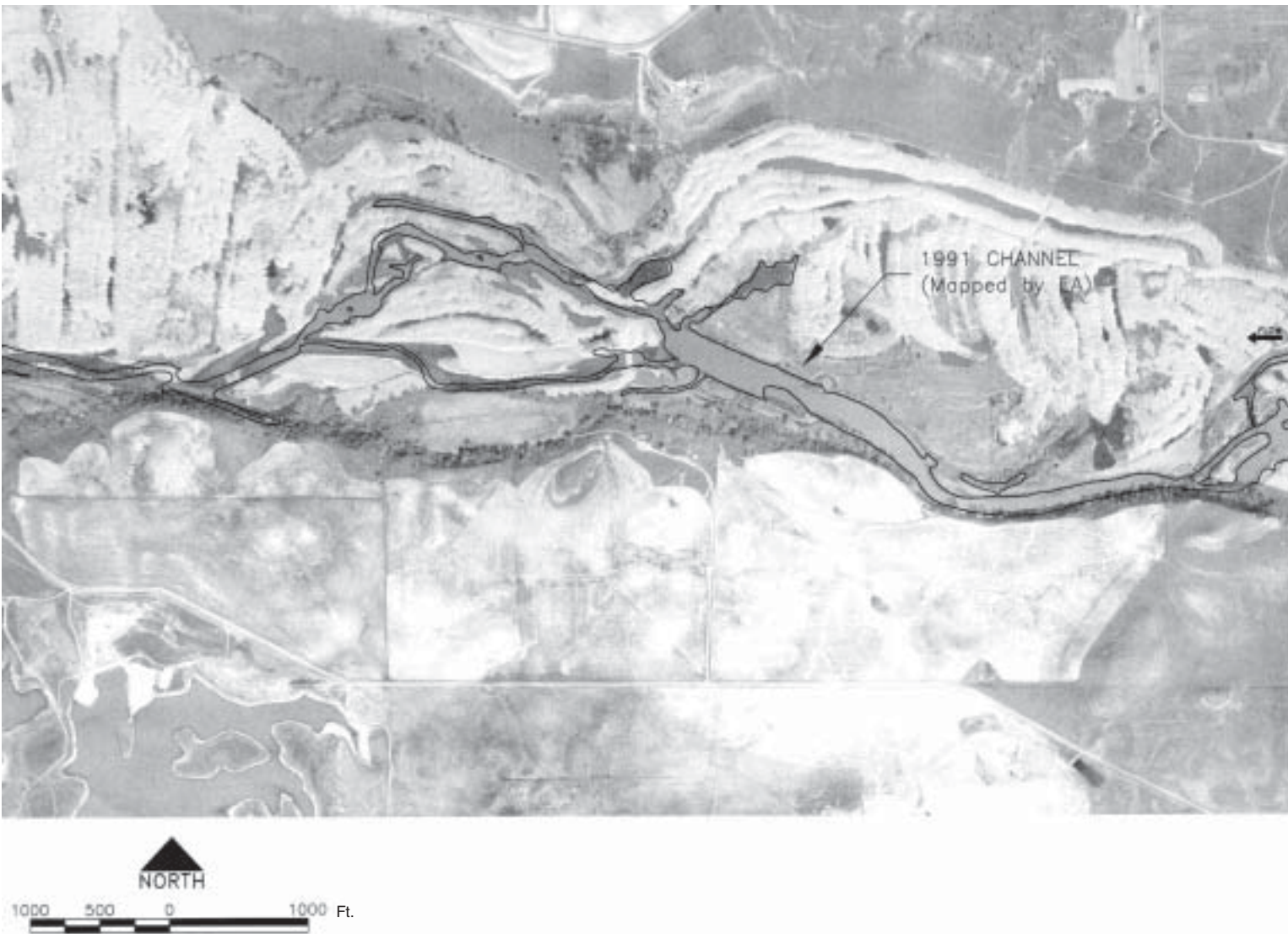
Figure 13. Dredge tailings upstream of Roberts Ferry (RM 43) in 1950 showing the impact of the dredge mining on channel morphology, and illustrating the static nature of the channel due to upstream flow and sediment regulation.
